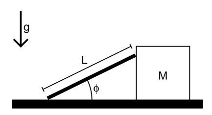
Find the forces on the rod immediately after the rod is placed in its initial position (at  $\phi = \phi_0$ ) and released.
