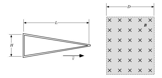
The point of the triangular loop enters the magnetic field at time t = 0. Graph the current induced in the loop as a function of time. Label the graph at all points at which the shape of the graph changes with the time and the current values expressed in terms of the given variables. Be sure to make clear which times the current is clockwise and which times it is counterclockwise.
