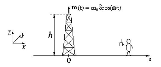
(a) Calculate the intensity of electromagnetic radiation at the ground level as a function of the distance from the base of the tower.
