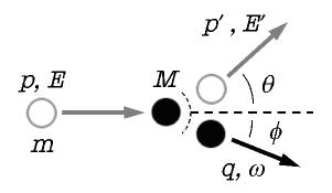
Consider the figure above and work in the *laboratory* system. A *non-relativistic* particle of mass m with energy E and momentum p collides with a stationary target of mass M. The incident particle scatters with energy E' (momentum p') at an angle  $\theta$ . The target particle recoils with energy  $\omega$  (momentum q) at an angle  $\phi$ .
