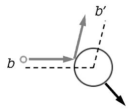
Finally, real particles have physical size and collisions are rarely *head-on*. The *impact* parameter b measures how far off the central axis the incident particle is. The same is true that the scattered particle trajectory will be parallel to but displaced by b' to a vector from the center of the target particle.
